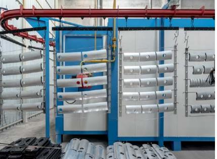
EPC (Electrostatic Powder Coating) - Metal
